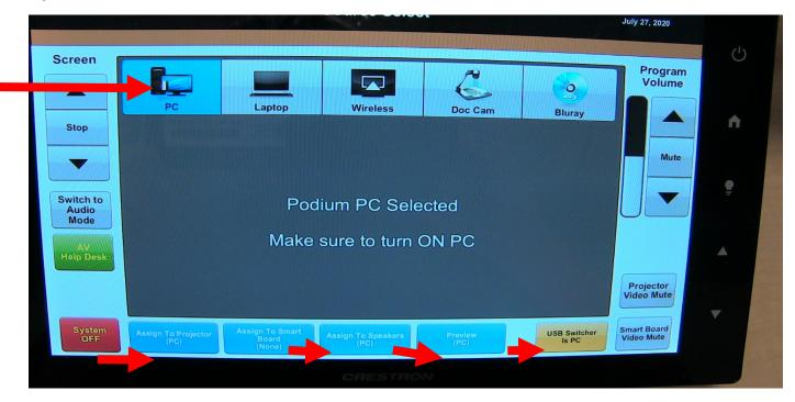
If a user wished to use their laptop select the laptop source from the top of the touch panel and assign it to the locations at the bottom of the touch panel, as shown below.
